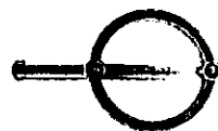
MBR200 Cast aluminum ring fixed to steel tube post, holds two bicycles. Custom raised lettering is available for ring. Weight: 29 lbs. (11 kg.)
